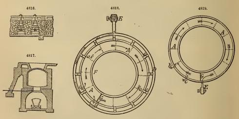
Figs. 4818, 4819, are sectional plans of a cheap construction of kiln intended to be worked on the continuous system, and specially adapted for the temporary use of contractors, or for erection on land containing only a thin seam of clay. In these modifications the construction of chimneys and smoke-chambers is rendered unnecessary, a forced combustion being maintained by the aid either of an exhauster or blower.
